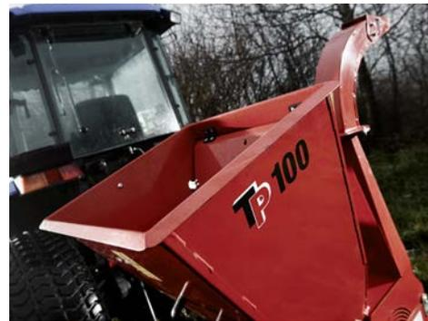
Owing to the vertical in-feed funnel, the TP 100 PTO is a compact machine that does not take up much space. The construction also enables a strong in feed without the use of feed rollers.
